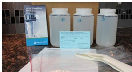
FIGURE 16: DENVER WATER'S 3-BOTTLE SAMPLING KIT
